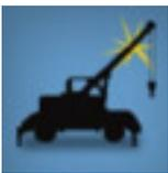
**High Reach Equipment**—Keep all cranes, scaffolding, and high reach equipment away from power lines. Contact with a power line can cause serious burns or electrocution. Remember to work a safe distance from all power lines. When performing construction activities, keep equipment at least 10 feet from power lines and 34 feet from transmission tower lines.
